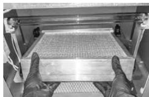
Make sure that the new hepa filter is properly fit in the filter frame. Otherwise, the device will not operate properly. The junked filters should be disposed properly and safely.
